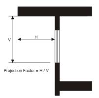
**Projection factor, side fin:** the ratio of the horizontal depth of the external shading projection to the distance from the window jamb to the farthest point of the external shading projection, in consistent units.
